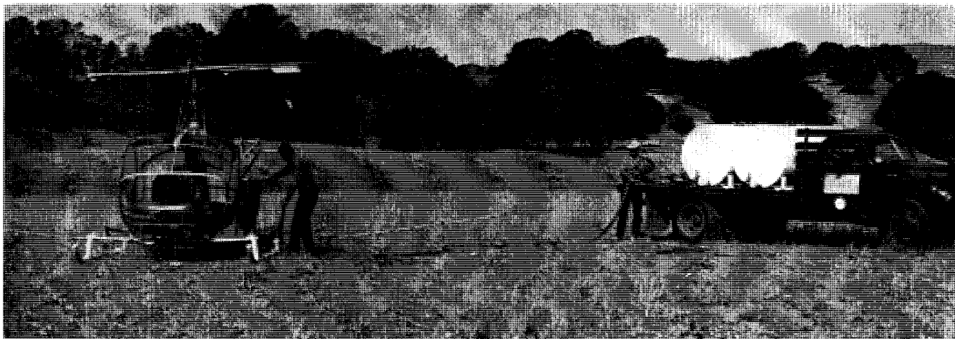
In California, helicopter is being tested for application of liquid fertilizers to rangeland. Nurse truck loads helicopter in less than a minute. Helicopter can reach land not accessible with ground equipment or airplane, and solutions stick without drift
